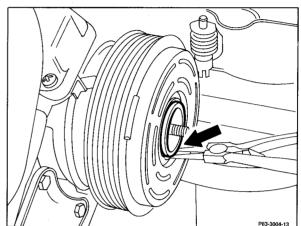
3 Replace bearing if required. Remove retaining ring from bearing (arrow).
