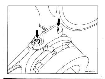
6 Remove snap ring on magnetic coil and remove coil.
