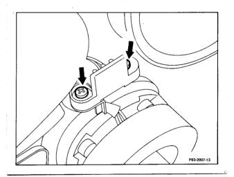
6 Remove snap ring from solenoid coil and remove coil.
