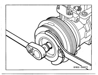
4 Screw puller into spring plate and pull spring plate.
