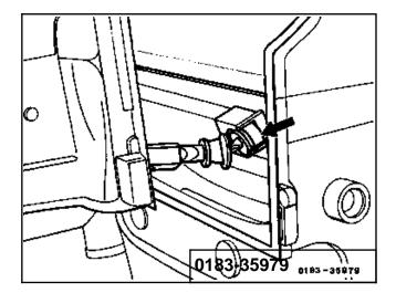
10 Unclip three clips (arrow) each on left and right side of heater and air conditioner box and remove upper section of housing.
