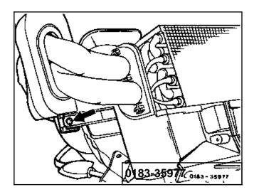
13 Pry evaporator (4) out of heater and air conditioner box.
