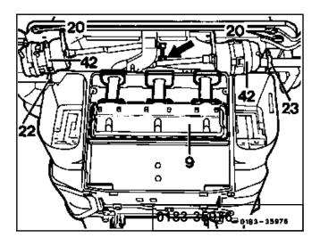
7 Screw out two screws (arrow) each on left and right side part.
