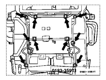
box downward and out after pulling outside air temperature sensor (B10/5) from holder.
