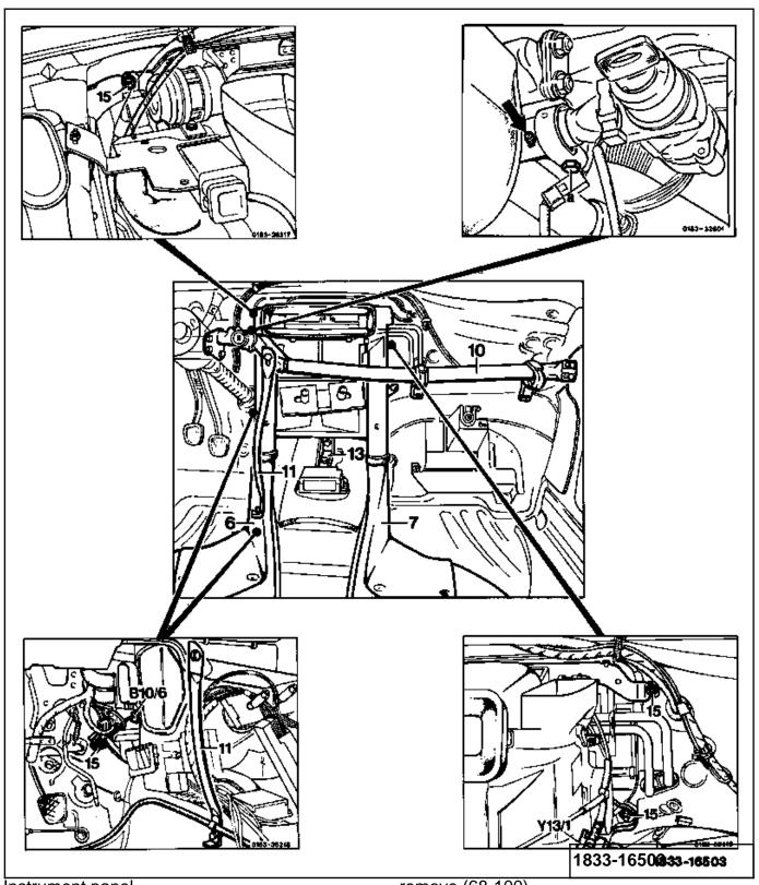
Instrument panel remove (68-100). Center console\_\_\_\_\_ remove (68-200). Left and right air duct (6 and 7) for rear
