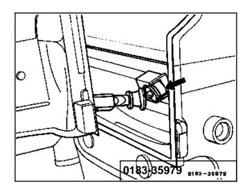
10 Unclip three clips (arrow) each on left and right side of heater and air conditioner box and remove upper section of housing.
