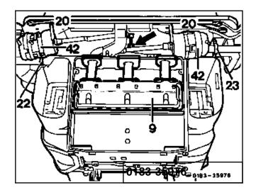
7 Screw out two screws (arrow) each on left and right side part.
