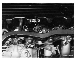
S25/5 Temperature switch 105/115 °C Model 124.0/2 with 6-cylinder engine
