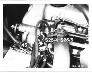
S25/4, S25/5 Temperature switch 100/110 °C and 105/115 °C Models 124.1/3
