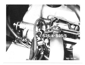
25/4 Temperature switch 100/110 °C Engine 601
