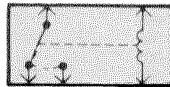
RELAY SHOWN WITH NO CURRENT FLOWING THROUGH COIL WHEN COIL IS ENERGIZED, SWITCH IS PULLED CLOSED
