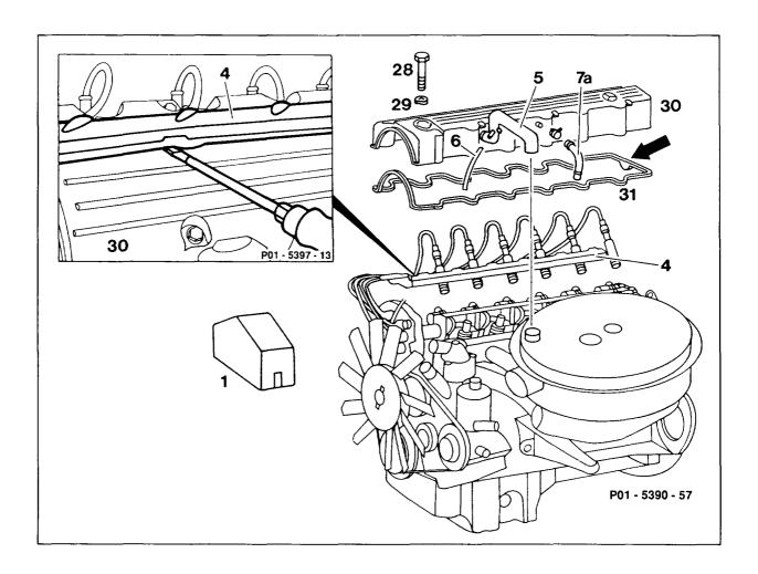
Cover (1) above high-voltage distributor unclip, remove, install.
