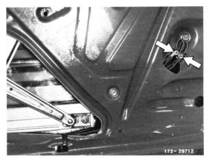
6 Unscrew nut on window lifting rail front and disengage window lifting arm.
