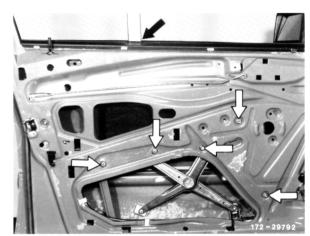
11 Insert window lift with motor and guide rail in door inside plate and fasten.
