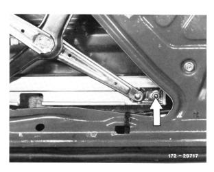
7 Lift window at the rear and extend slide shoes at cutout of window lifting rail.
