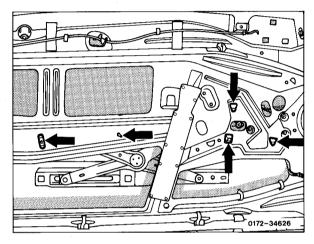
11 Rivet window lift to inside door plate with riveting tongs and blind rivet dia. 6 mm (3 each).
