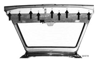
Unscrew fastening nuts for wiper motor.
