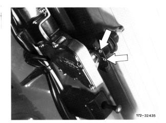
6 Separate connections for heatable back window pane at left and right on tailgate.
