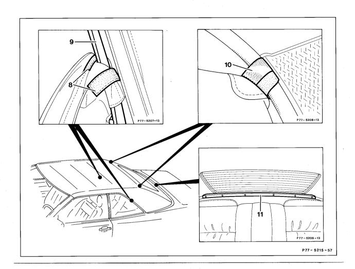
Velcro strip (8) on main pillar (9)open, close (item 8).Velcro strip (10) on corner braceopen, close (item 5).Cover (11) on soft top bowremove, install.Headliningdetach from, glue onto soft top bow (item 16).
