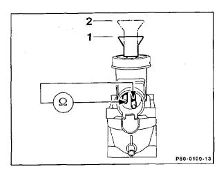
Testing opening function of actuator.
