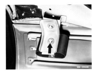
2 Unscrew both fastening nuts left and right on side member.
